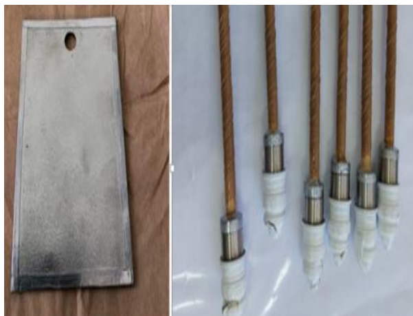
Figure 1: View of the standard plate and shroud-fuel nozzle prepared for the hard chrome plating process
