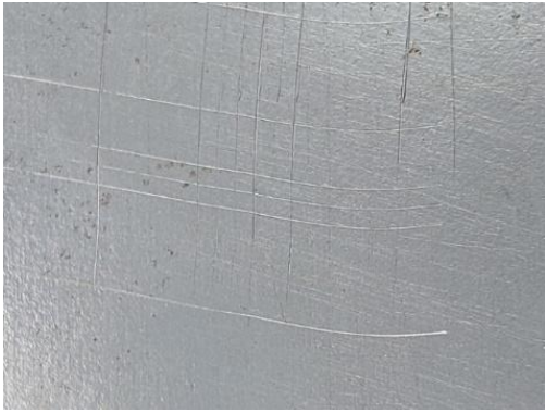
Figure 5: The appearance of the plate examined by the notch method
