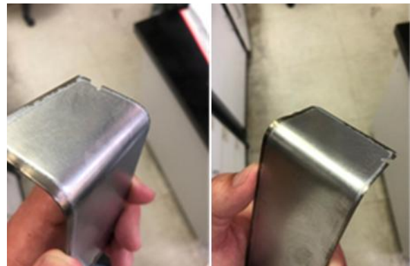
Figure 4: The appearance of the plate after bending at an angle of 90°
